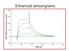
EpiGrammer can also split the original sensorgram data into two separate channels, each channel being specific for one of two different binding species. One channel – the 'epigram' – is specific for the dyelabelled species, while the other channel – the 'ektogram' – is specific for any unlabelled species:
